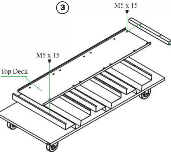
1. Using M5 bolts attach the Top Deck onto the Y-shape Decks
