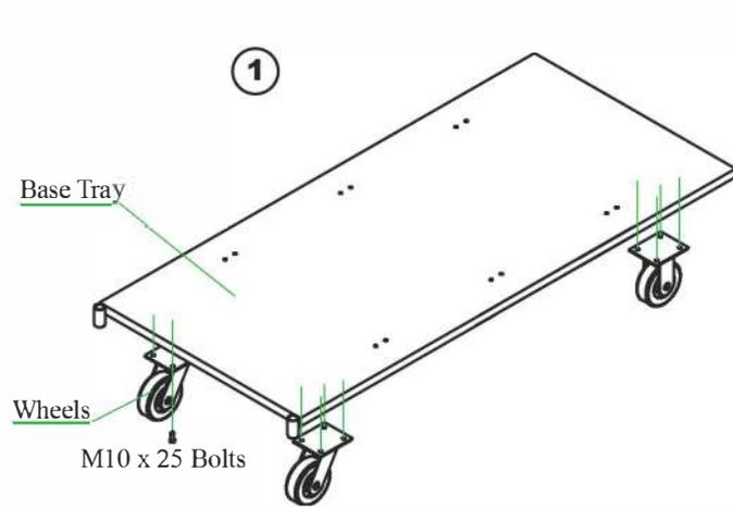
1. Attach the 4 Wheels to the bottom of the Base Tray using the M10 bolts making sure the wheel plates are facing in the correct direction
