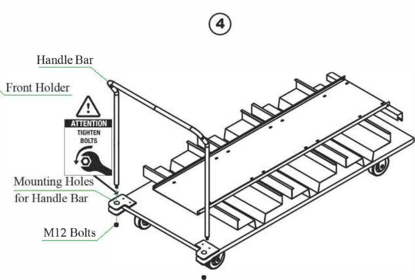
1. Place the Handle Bar inside the mounting holes on the Base Tray
