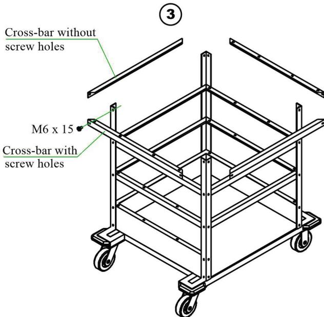
1. Using 2 x M6 bolts attach the cross bars onto the uprights
