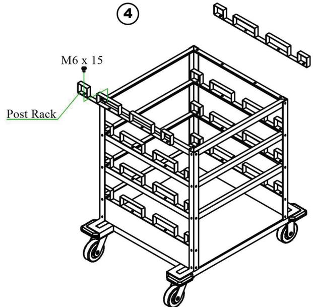
1. Using 4 x M6 bolts attach each Post Rack to the Cross Bars NOTE: Keep these bolts loose
