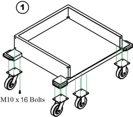
1. Attach 4 Wheels to the bottom of the Storage Tray using the M10 bolts making sure the wheel plates are facing in the correct direction
